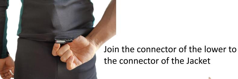
The connector of the jacket is at the bottom of the back as shown in the figure
